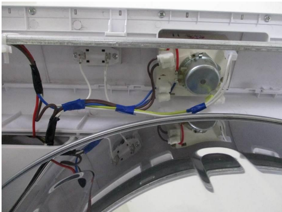
Switch for heater and timer switch (T90-1)
